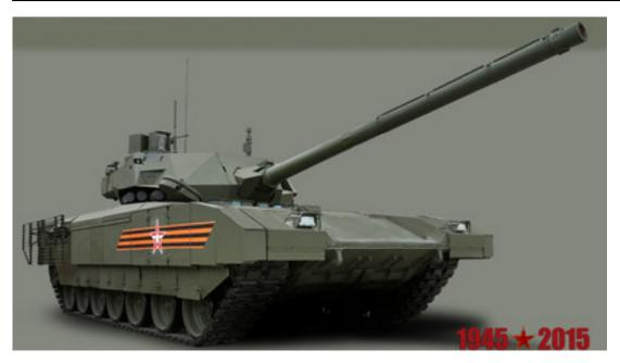
The Armata's main advantage over similar existing technology lies in its unmanned turret, controlled remotely from an isolated armored capsule. The latest tank has a state-of-the-art radar system that can simultaneously track up to 40 ground and 25 air targets within a 60-mile (100km) radius.
